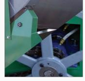
Drum rollers are lubricated from the front of the mixer / Some bearings have remote grease zerks
