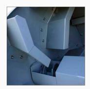
Oversized scoops are secured with stainless steel hardware allowing them to be replaced when required.
