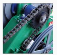
A super strong, quiet synthetic idler for the main drive chain is fully adjustable, while the drum drive utilizes a springloaded idler. All bearings have grease fittings for maintenance.
