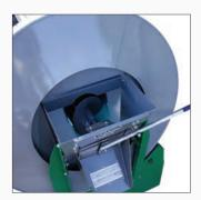
Standard on each model are magnets on the chute and an efficient, easy to operate manual discharge door.
