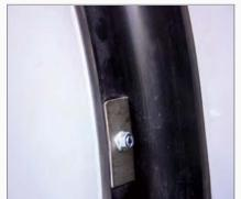
Passive ribs (see arrows in above cut out) disturb the outside of the feed load creating a secondary mixing action. All parts that come in contact with feed are finished with a 'stick resistant' super strong epoxy powder coating. To reduce clatter, heavy wall PVC pipe is used to encase the auger. Its practical, efficient and cost effective.
