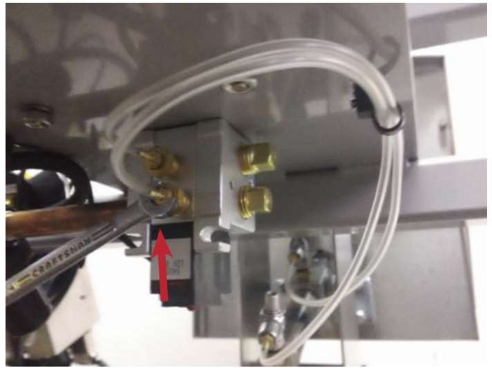
Fig. 6: Unscrewing the brass barbs holding the hoses to the solenoid
