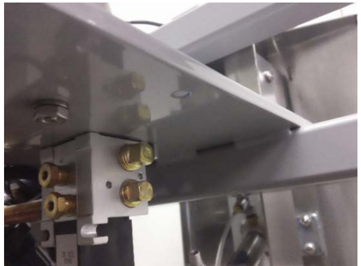
Fig. 7: Solenoid and chassis without air hoses attached
