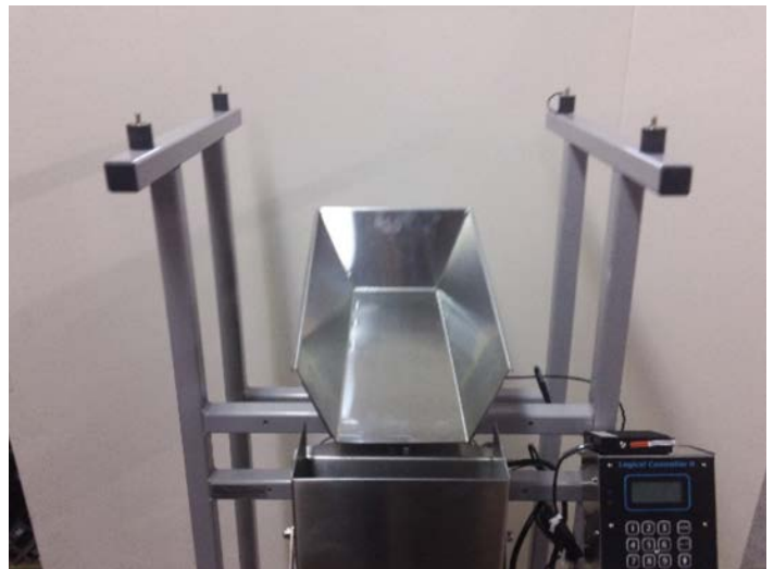
Fig. 2: Feed Pan exposed after removing Supply Hopper
