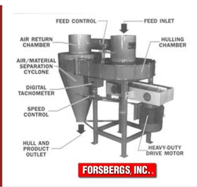
The product is fed into the inlet where it enters the impeller wheel through the feed control pipe. Accurate crank adjustment of the feed control determines the thoroughness of the hulling operation. The centrifugal force of the rotating impeller wheel drives the product against the hulling ring. Both the impeller and hulling ring are constructed of a durable boralloy steel for wear resistance.
