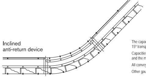
The capacities shown are for conveyors with a maximum incline of 15° transporting free-flowing dry material at 45 lb./cu. ft. or 56 lb./bu.
