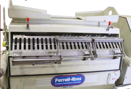
Ferrell-Ross offers magnet assemblies as an option on all its industrial roller mills. This magnet is designed to capture ferrous tramp metal contaminants from the product stream before passing through the rolls. This assembly then allows easy cleaning of the magnets simply by opening the feeder door.
