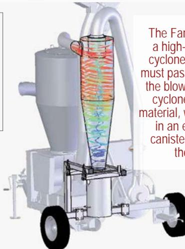
The Fan Guard utilizes a high-efficiency dust cyclone in which the air must pass before entering the blower housing. The cyclone removes fine material, which is collected in an easily emptied canister directly under the cyclone.
