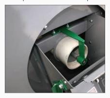
To reduce clatter, heavy wall PVC pipe is used to encase the auger. It's practical, efficient and cost effective.
