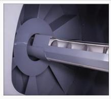
Huge scoops pick up the ration and dump it into an auger that moves the feed forward. With the discharge door closed, the feed drops into the drum and moves to the back for the process to be repeated. A removable cover provides access to the auger.
