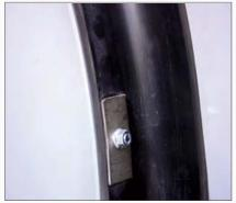
Passive ribs (see arrows in above cut out) disturb the outside of the feed load creating a secondary mixing action. All parts that come in contact with feed are finished with a 'stick resistant' super strong epoxy powder coating. To reduce clatter, heavy wall PVC pipe is used to encase the auger. Its practical, efficient and cost effective.
