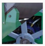
Drum rollers are lubricated from the front of the mixer / Some bearings have remote grease zerks
