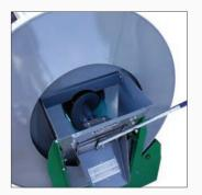
Standard on each model are magnets on the chute and an efficient, easy to operate manual discharge door.
