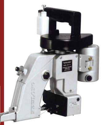
The NP-7A has a robust construction for reliable operation with minimal maintenance. Specially designed features extend the life of the equipment; plastic shock resistant isolation handle, automatic oiling system for lubrication of moving components, extra wide feed dogs, automatic thread cutting and our improved steel cam.
