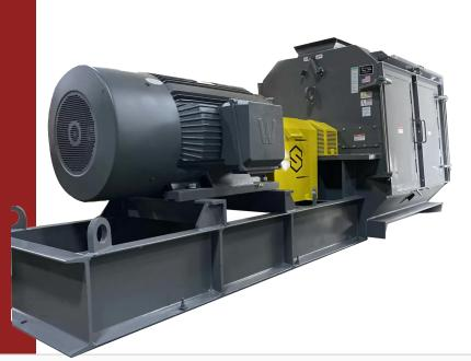
The 44 Series hammer mill is designed for very high production grinding of agricultural products, feed and grain, light wood waste and other relatively easy to grind materials. The nearly full circle screen translates to a larger open screen area and thus the highest possible production rates on materials that do not require initial grinding against a breaker plate.
