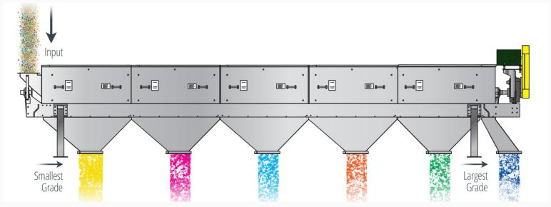
The Gentle Roll™ Standard Model offers a wide range of models and configurations. The flexibility of the design allows you to remove fines, overs, fines & overs, or separate by size.
