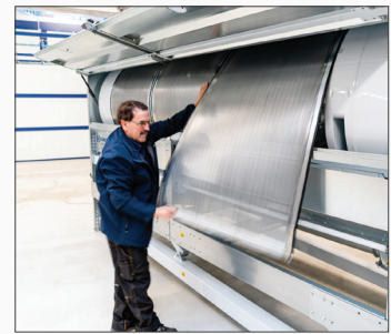
Quick-release system makes it easy to change screens and prepare for the next crop.
