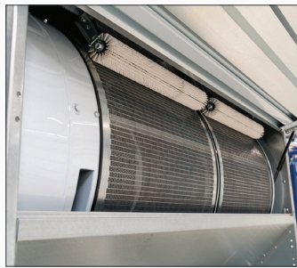
Cleaning brushes are mounted on a spring-loaded arm for efficient even load on the outer screens.
