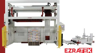
STACKING RECIPES ARE EASY TO MAKE AND CAN BE QUICKLY CHANGED BY THE OPERATOR. **EZRATEK OFFERS COMPLETE BAG INFEED LINES WITH A BAG** TURNER OR A BAG KICKER.
