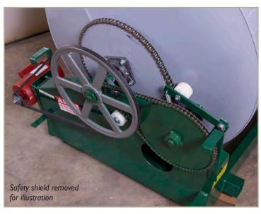
All bearings have grease zerks and are easily accessed for replacement when required. A quiet, long life neoprene roller is used in the spring-loaded idler to assure maximum efficiency and extended drive chain life.
