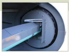
A heavy 3/8" thick neoprene seal keeps feed in the drum where it belongs.
