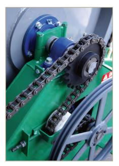
A super strong, quiet synthetic idler for the main drive chain is fully adjustable, while the drum drive utilizes a springloaded idler. All bearings have grease fittings for maintenance.
