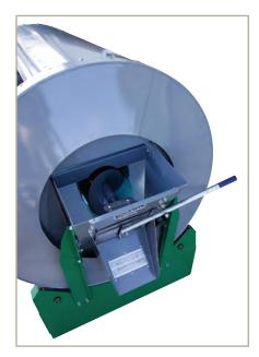
Standard on each model are magnets on the chute and an efficient, easy to operate manual discharge door.
