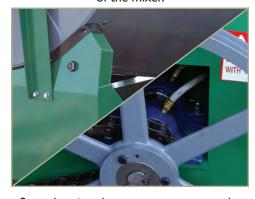
Some bearings have remote grease zerks
