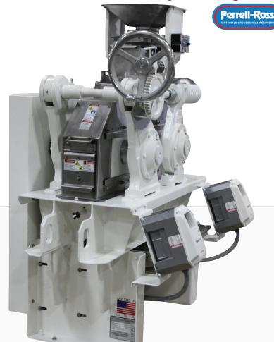
The Ferrell-Ross 18x6 Laboratory Flaking Mill is extreamly versatile and an ideal choice for labratory, R & D or pilot plant settings. With the inverter duty motors and controls you can easily change roll speed and differential often reqired for labratory and R & D applications by simply adjusting the inverter setting.
